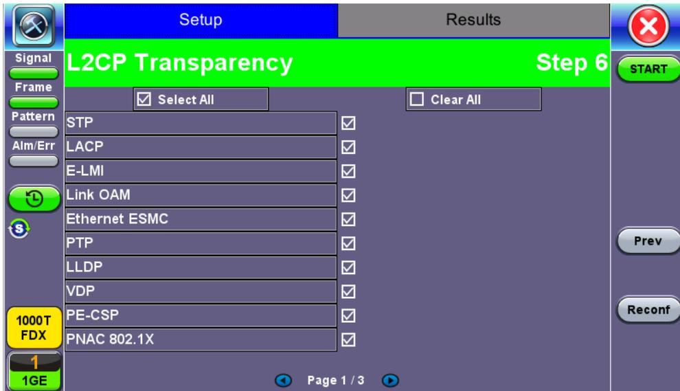
L2CP Transparency Test - Transmitter - Step 6
